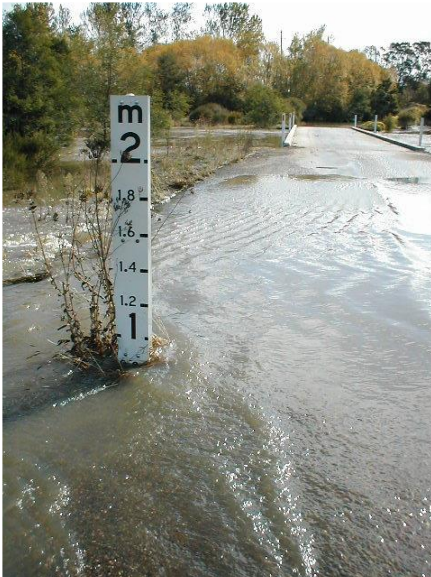
Figure 5-2 Typical Flood Depth Marker Sign 1
